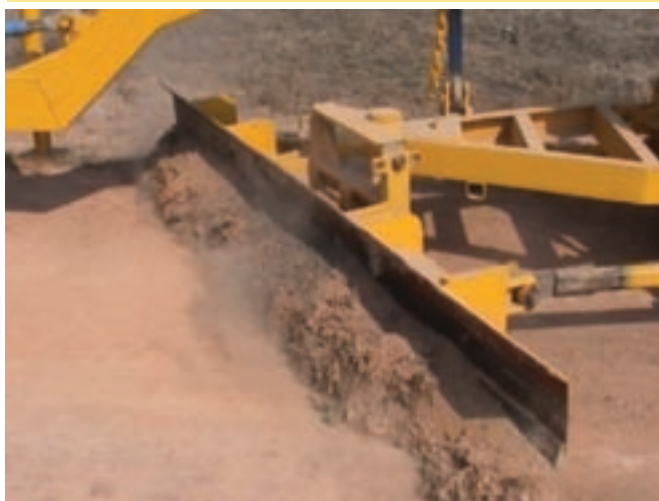
Figure 4 - ENGINEERED NATURAL SURFACES: Maintainable using simple locally made equipment
